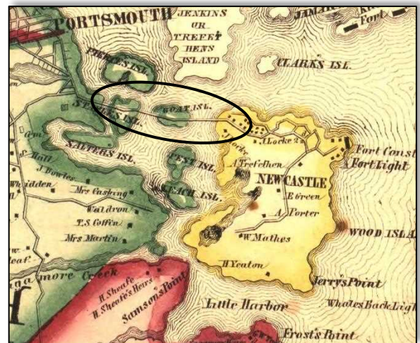
Portsmouth-Newcastle Bridge on the 1858 Chase map, originally consisted of three pile trestles. The middle trestle had a bascule-type draw, removed in 1941.
