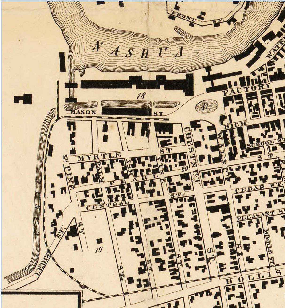
FIGURE 7: 1858 map of Nashua, showing further development of Nashua Manufacturing Company mill complex, most importantly the addition of the Worcester & Nashua Railroad serving the mill with a line that runs north along the canal after branching off the main line along Hollis Street. A low stone retaining wall was built along the east side of the canal to support the bank alongside the railroad tracks. Based on a comparison to the 1842 map (Figure 6) the canal appears to have been realigned more due-north, but the difference may be a mapping inaccuracy. The tracks then extend over the Canal Basin on a new bridge (see Figure 8) and east along Basin Street. Three bridges now span the Canal Basin. (Source: Chase 1858).
