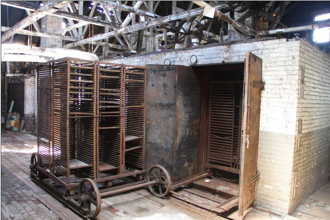
Photo No. 23: Paint Shop, interior, Drying Ovens, showing custom designed trolley and unitized drying racks. Present and labeled "Japan Ovens" on 1898 Sanborn map. Looking E.
