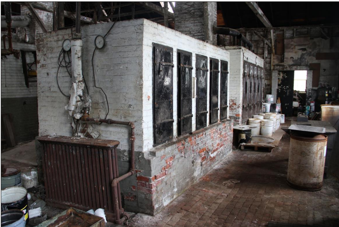
Photo No. 24: Paint Shop, interior, showing another type of Drying Oven. Present and labeled "Japan Ovens" on 1898 Sanborn map. Looking S.
