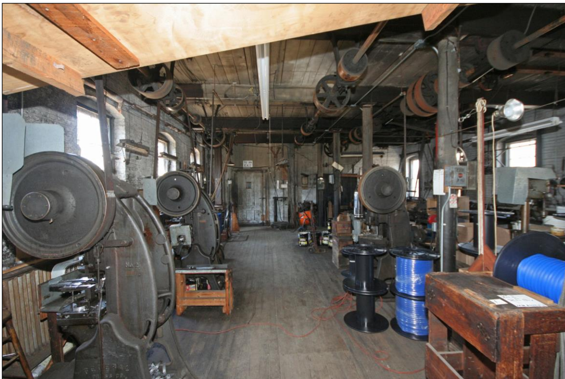
Photo No. 21: Factory, interior, Button Machine Shop, showing original overhead line shafts and belt driven machinery. Looking W.
