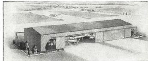
Fig. 470 (above). Butler (All-Steel) Type MT Hangar. This multiple unit hangar is designed for 4 planes but can be increased in accordance with requirements: 30' wide, 118' long and 12' high with 9' clear opening door.
